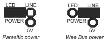
Fig.3 Jumper POWER - Power source configuration
